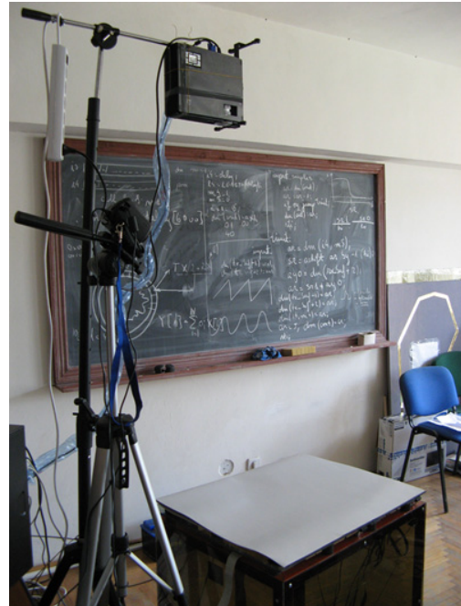
Figure 4. Prototype installation of equipments: video projector and tabletop with installed sensors. The projector images are automatically computed by a desktop PC in accordance with the data received from the tabletop via the serial connection.
