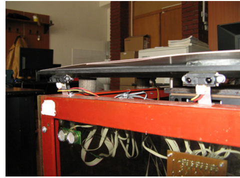
Figure 3. Tabletop prototype: installation of short-range sensors around the table (two sensors in view: middle and corner installed on the same edge).
