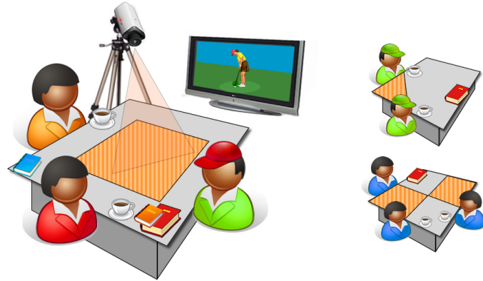
Fig. 1. Left: our vision for interactive coffee tables: all the viewers may interact with the TV set using the same wide-area interface via simple hand movements on top of the video-sensitive area of the table. The interactive area is depicted in the center of the table by using a darker color. Right: Several possible designs for the interaction sensitive area on the coffee table accommodating for 2 or multiple viewers.
